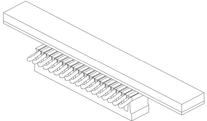
Figure 1. Linear motor configured as a short stator
