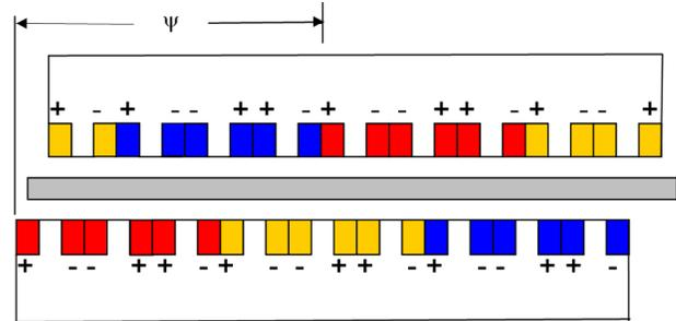
Figure 7. Machine using 9 coil 8/10 pole stators
